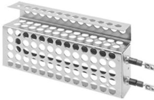
When installed, the strip heater is used to maintain the internal enclosure temperature above ambient conditions to help reduce the effects of condensation and moisture.
