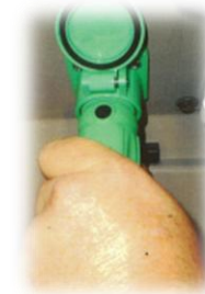
Tug lightly to verify secure engagement.
