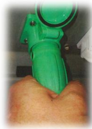
Grasp Cam-Lok firmly and rotate counterclockwise until it stops.
